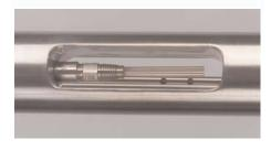
The voltage output from each sensor and bridge board set is sent to its own microprocessor board for accurate linearization of the flow rate signal. The linearized output signals from the multiple sensors in
