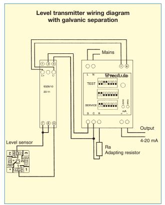
The adapting resistor value should be ten times the resistance of the level sensor at minimum level. Normally the level sensors have a resistance of 1000 ohms/meter and a 2,5 meter long level sensor would have an adapting resistor of  $25k\Omega$ . On demand communication with HART, Profibus of Fieldbus protocol.
