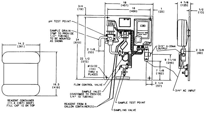
THE NUMBER OF CONTAINERS AND REAGENT PUMPS PROVIDED, DEPENDS ON THE TYPE OF RESIDUAL BEING MEASURED, AND THE METHOD OF PH CONTROL ( ACETIC ACID OR CO2 ).
